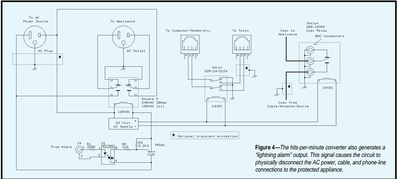
**Figure 4**—The hits-per-minute converter also generates a “lightning alarm” output. This signal causes the circuit to physically disconnect the AC power, cable, and phone-line connections to the protected appliance.
