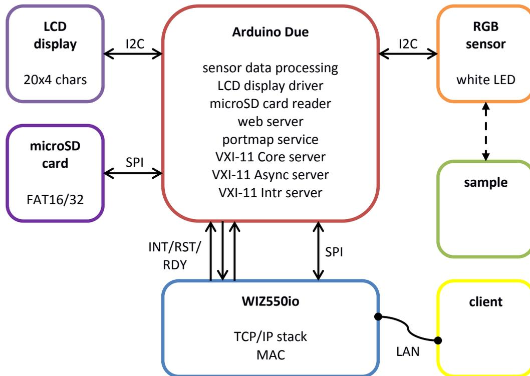
Figure 1, block diagram of the Instrument of Things.
