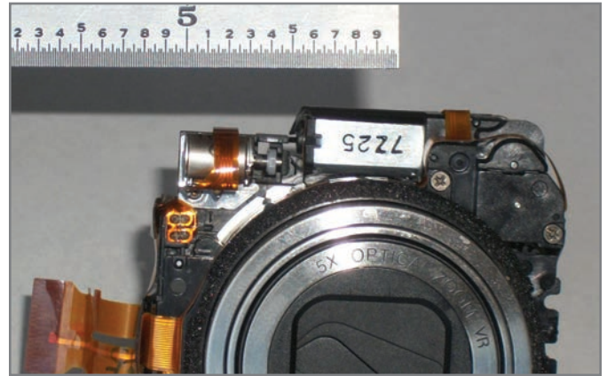
Photo 3 —Top view of the horizontal sensor-shift actuator. At the top left corner is one of the smallest stepper motors I have ever come across, only 0.3" long. It has an internal leadscrew to move its shaft horizontally, which presses against a carriage to move the image sensor. The larger motor to its right controls zooming and lens retraction.
