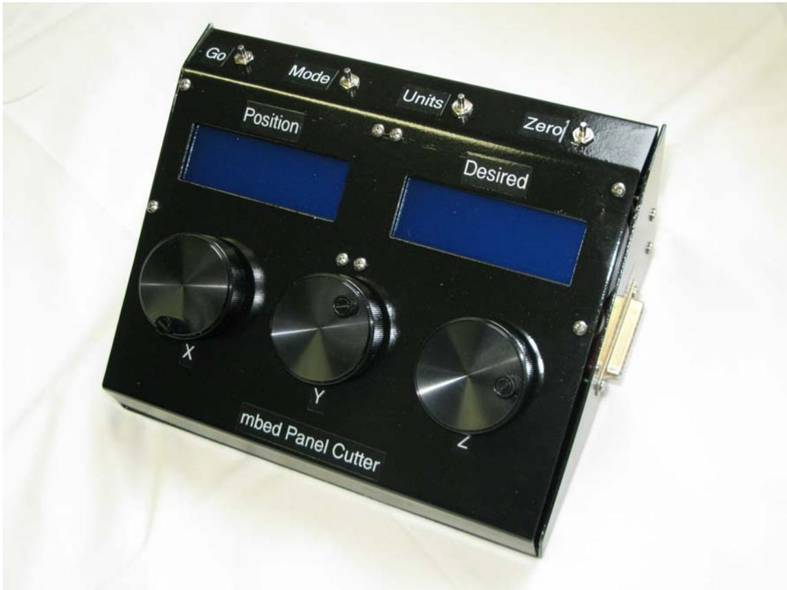
Figure 2 Photo of the completed controller. The front panel was cut using this system.
