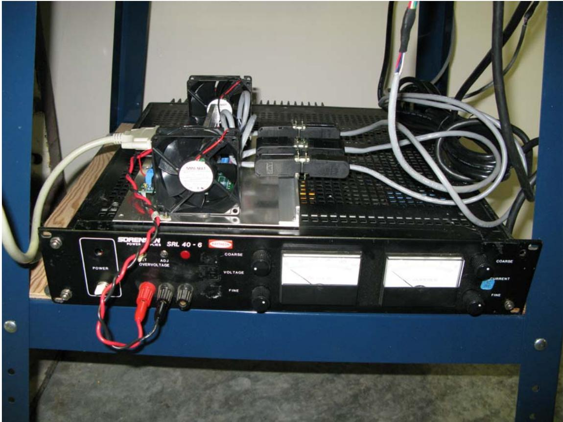
Figure 4 Sorensen power supply with HobbyCNC board on top. This is on a shelf under the milling machine.
