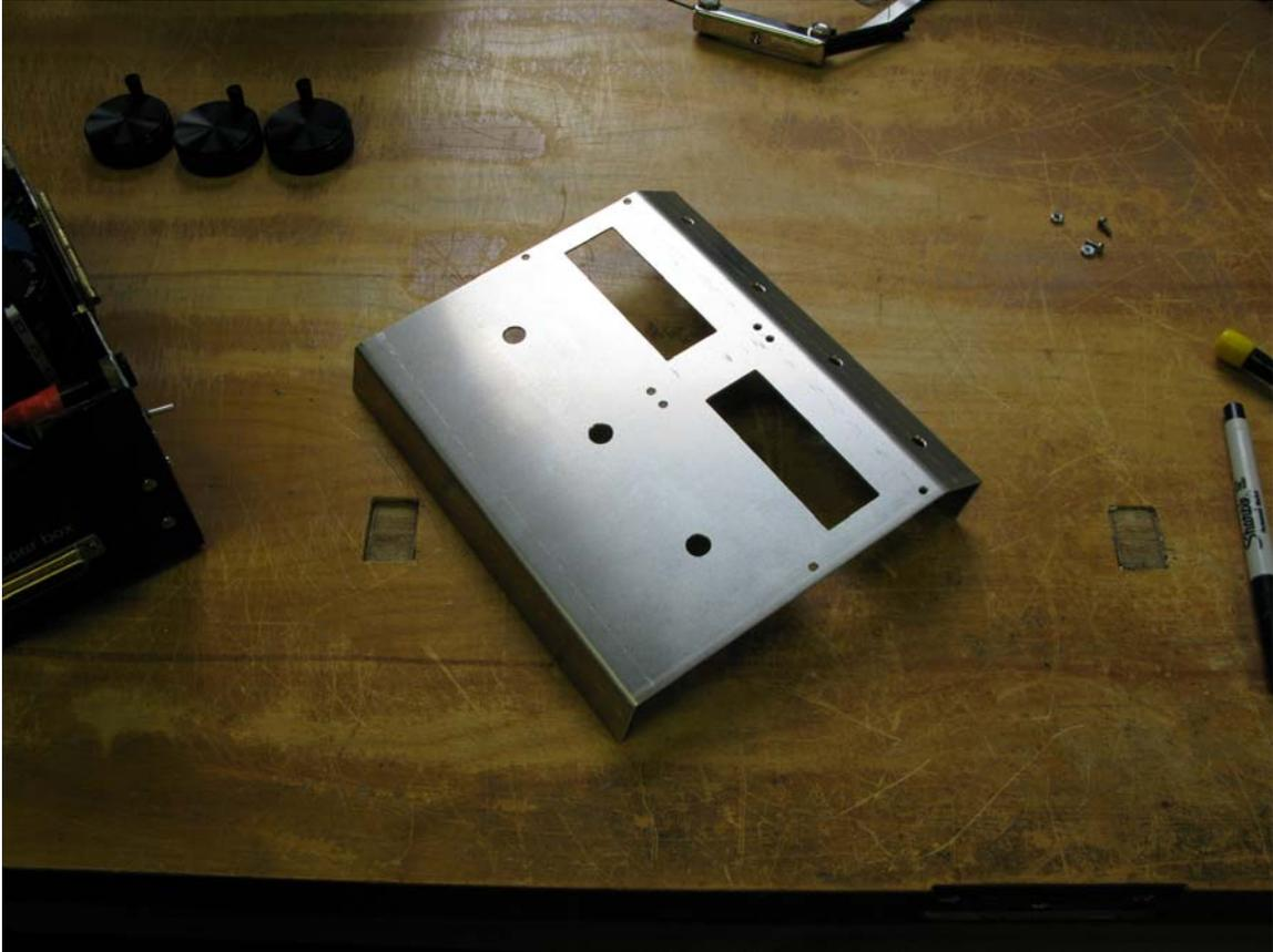
**Figure 8 Front panel after bending**
