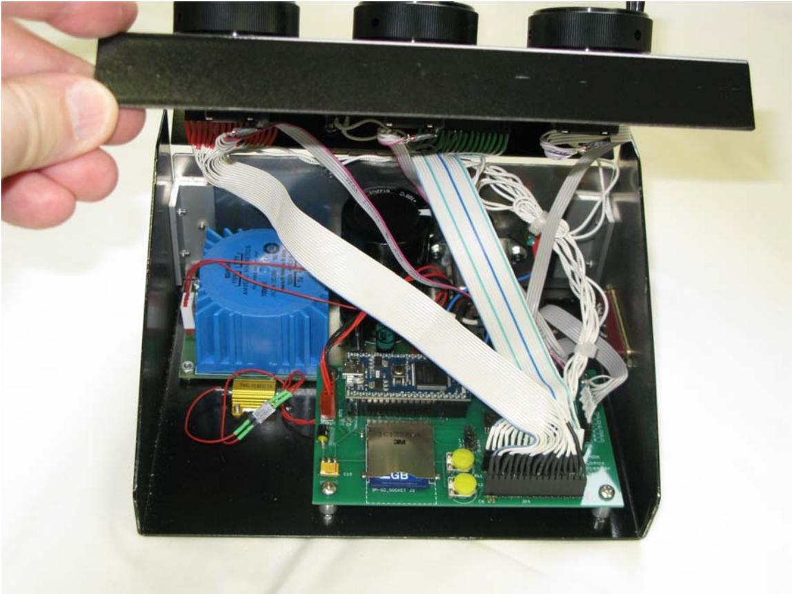
Figure 9 Photo of the controller with the hinged front lifted up to show power supply and printed circuit board holding the mbed module. Having a hinged front panel allows easy access to the SD card.
