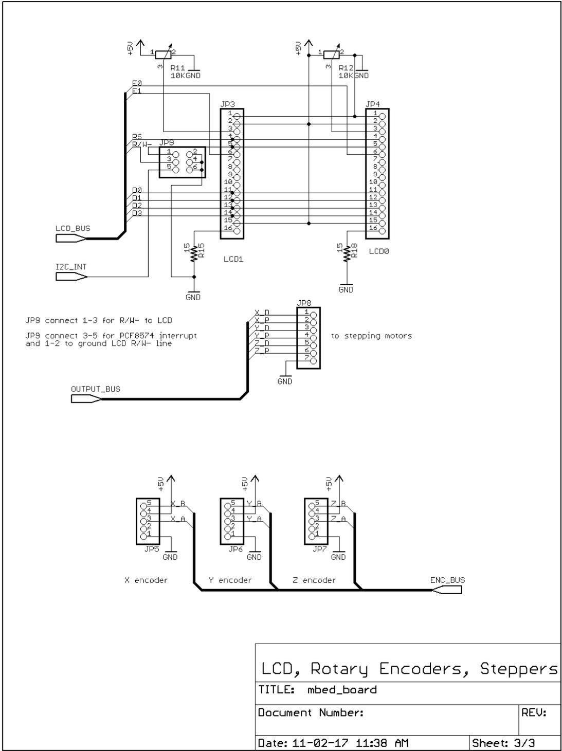
Figure 5c Encoder, output and LCD connections
