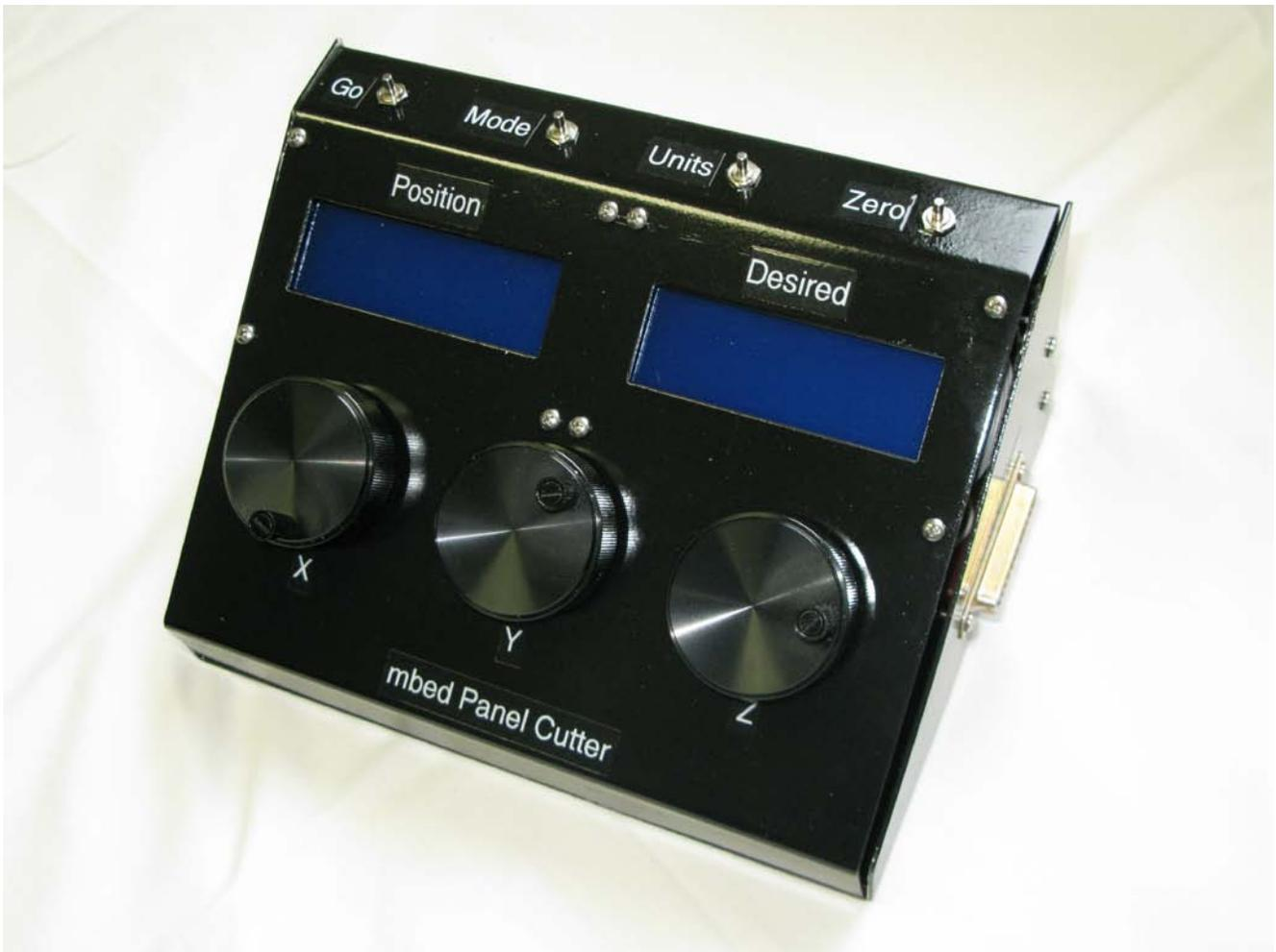
*Figure 1 Photo of the completed controller. Its finished panel was cut using the system.*
