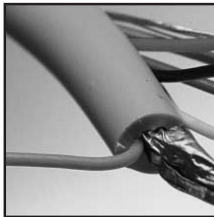
**Photo 3**—This section of PS/2 keyboard cable shows the insulated conductor molded outside the shielding foil. A keyboard wouldn't notice, but a microphone might misbehave.
