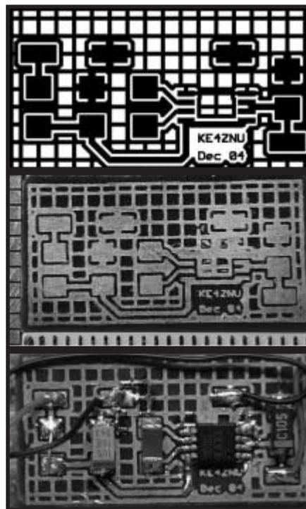
**Photo 1**—The top image is the top copper layer from an EAGLE board design. The bare board shows several flaws, but the one on the bottom came out fine. The ruler scales are 0.050" vertically and 1 mm horizontally. The board has extremely small features!
