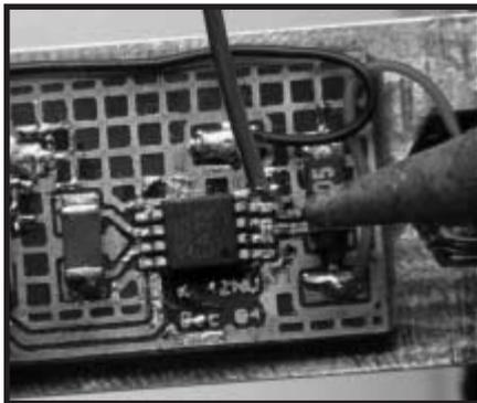
**Photo 2**—Hand-soldering SMD parts is possible if you learn some new techniques. First of all, the board must be horizontal so the parts don't slide off!
