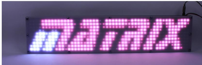
large number of LEDs. Again the Flowcode component offers full simulation and also compatibility with the Bitmap Drawer component allowing us to easily display and animate the Matrix logo as seen in **Figure 5**.
