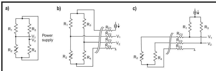
**Figure 1a**—Here the bridge circuit has one variable element. **b**—In this instance, all four bridge components are found in the soldering pen. It's the most obvious way of adding a cable to the circuit. **c**—The new circuit topology involves a cable with only three conductors to complete the bridge circuit.
