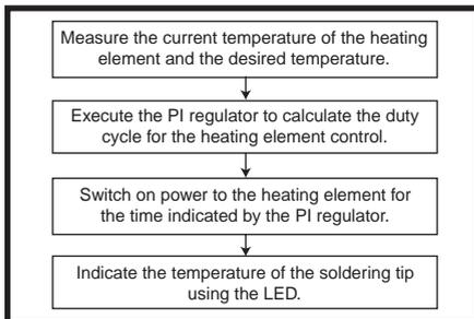
Figure 5—The microcontroller executes this algorithm repeatedly in an endless loop.
