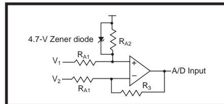
**Figure 3**—An op-amp is used to create the differential amplifier that amplifies the voltage across the bridge circuit. The Zener diode protects it against overvoltage when the heating element is on.
