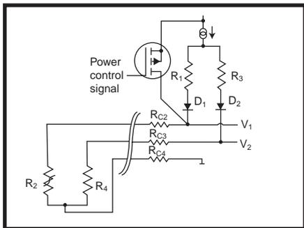
**Figure 2**—It's a fairly simple solution, right? Simply add the power switch and protection diodes.
