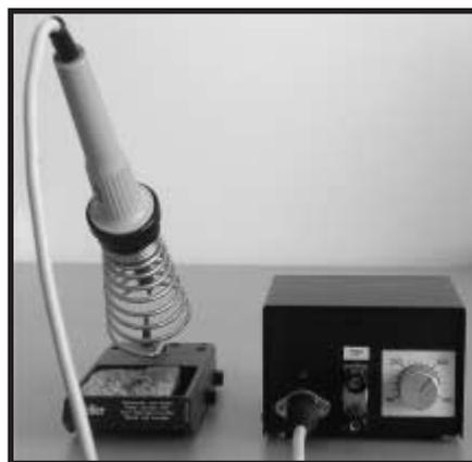
**Photo 1**—Check out my finished soldering station. Think of it as a heating element turned temperature sensor.
