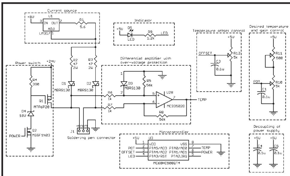
**Figure 4**—The power supply is the only part not shown in the schematic of the soldering station. The current source is powered by 8 V to reduce power dissipation.
