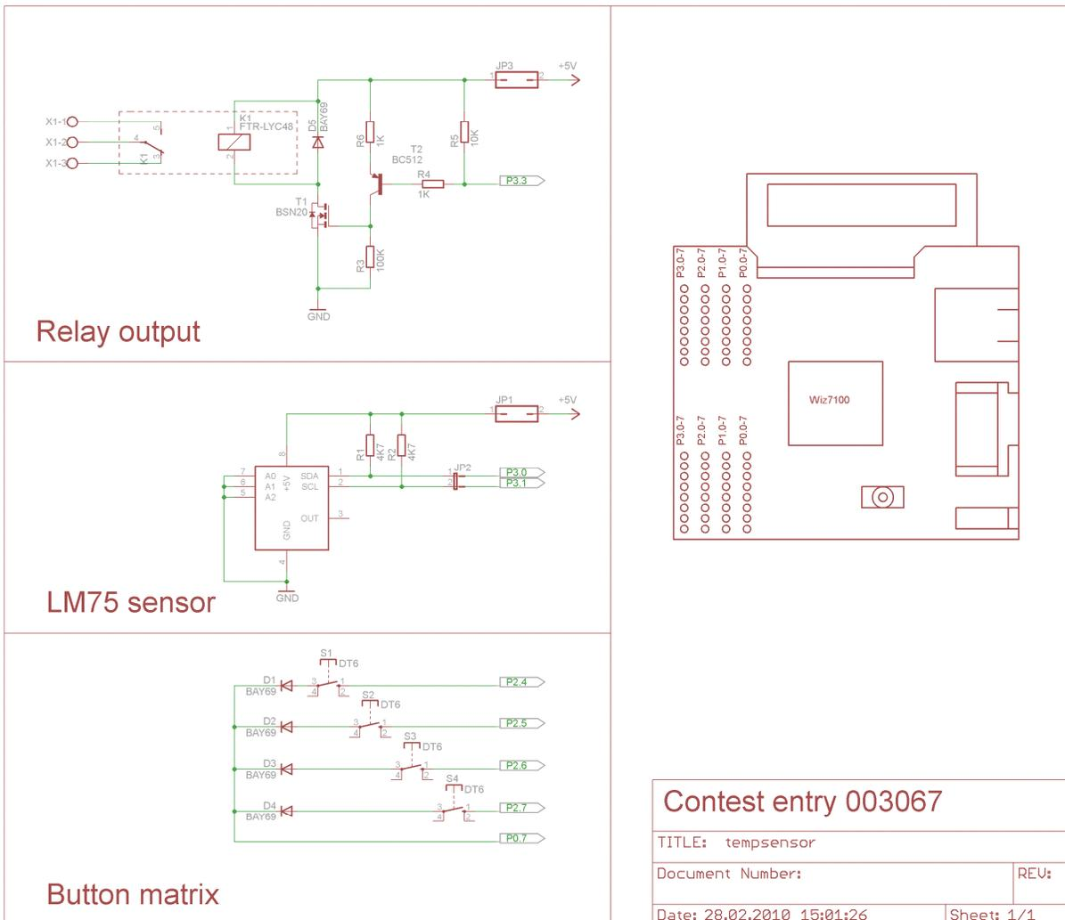
Figure 3: Schematic of extensions to the WIZ7100 evaluation board.
