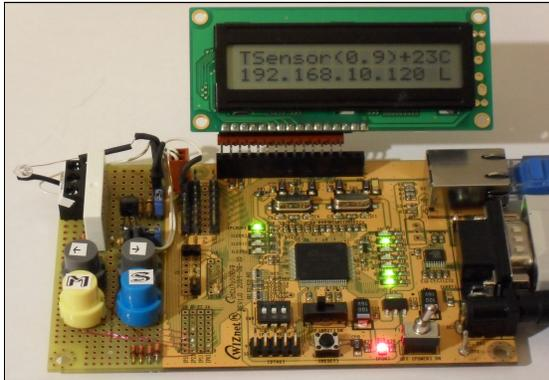
Figure 1: Prototype hardware based on the WIZnet evaluation board.
