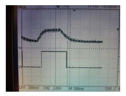
The signal showed in channel two is the signal after an amplifier, a low pass filter and finally a comparator implemented with an operational amplifier LM339.
