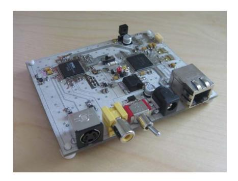
At its core, the UPnP Picture Viewer is powered by a WIZnet W7100 Internet MCU. The W7100 is an integrated networking solution, combining a
