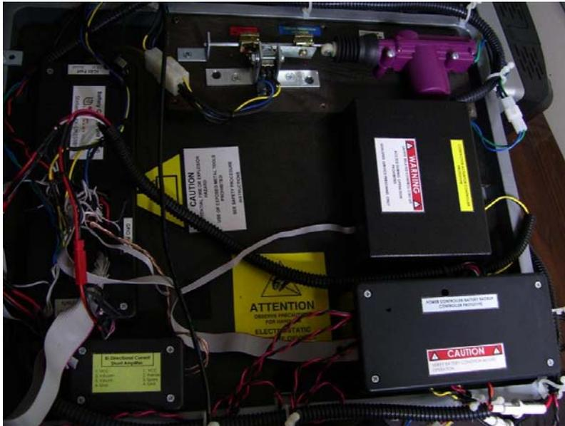
Figure 4. The top view: the various custom prototype hardware boards, in their enclosures, as required for operation. Top: circuit protection contactor (functional model); middle right: actuator controller board. Lower right: power controller board. Lower left: current shunt monitor board. Upper left: the Stellaris-based BCU board in its enclosure & wiring.
