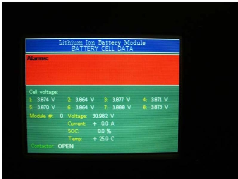
Figure 3. The LCD monitor displaying module parameters including cell/ambient temperature, load current, individual cell voltages, total module voltages, real-time contactor position (open or closed), and any alarms as they appear. Note that the StellarisWare GRLIB graphics library is used to draw graphics and text. Custom drivers were developed to control the Solomon Systech SSD1963-based LCD driver board
